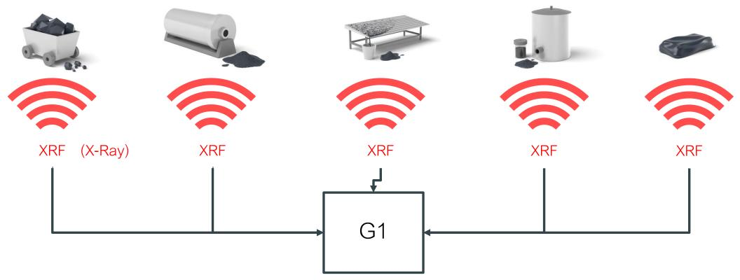
XRF: Rapid X-ray fluorescence that yields the elemental distribution. Between 5 and 500 measurements per product needed.
